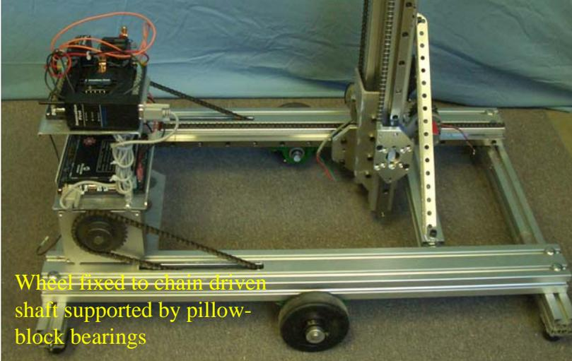
Wheel fixed to chain driven shaft supported by pillow-block bearings
