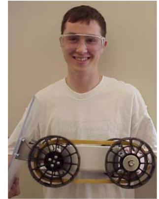
Nick Powley obtained 4WD by cutting grooves in his wheels and using rubber bands as drive belts...
