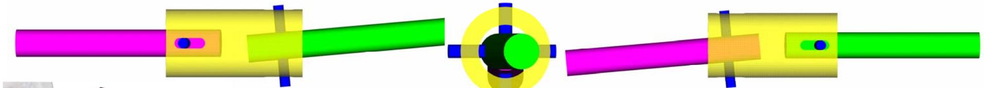
***Critical: Note the clearance between the coupling bore and both shafts!***
